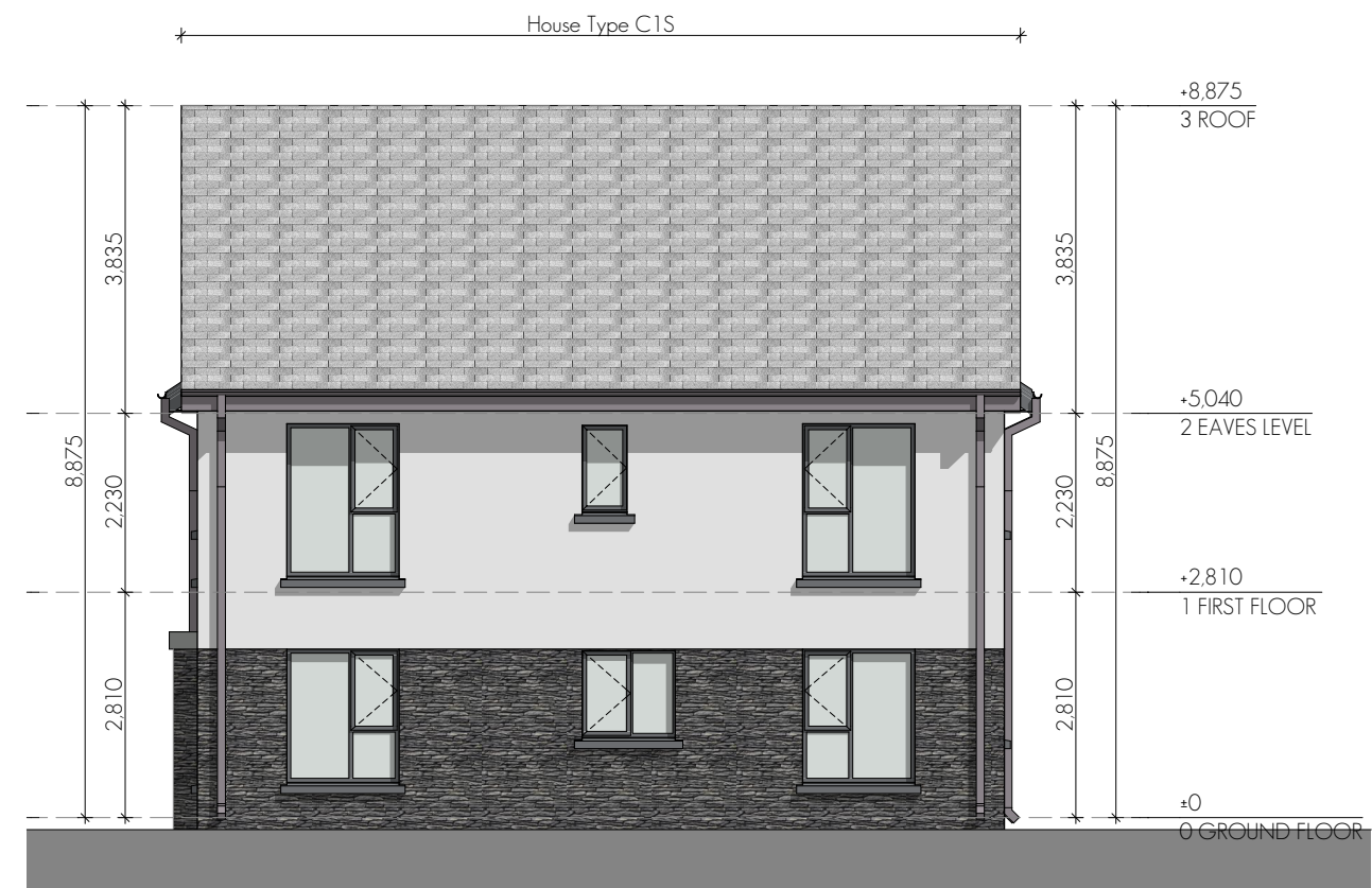
B GABLE ENTRY ELEVATION 1:100
