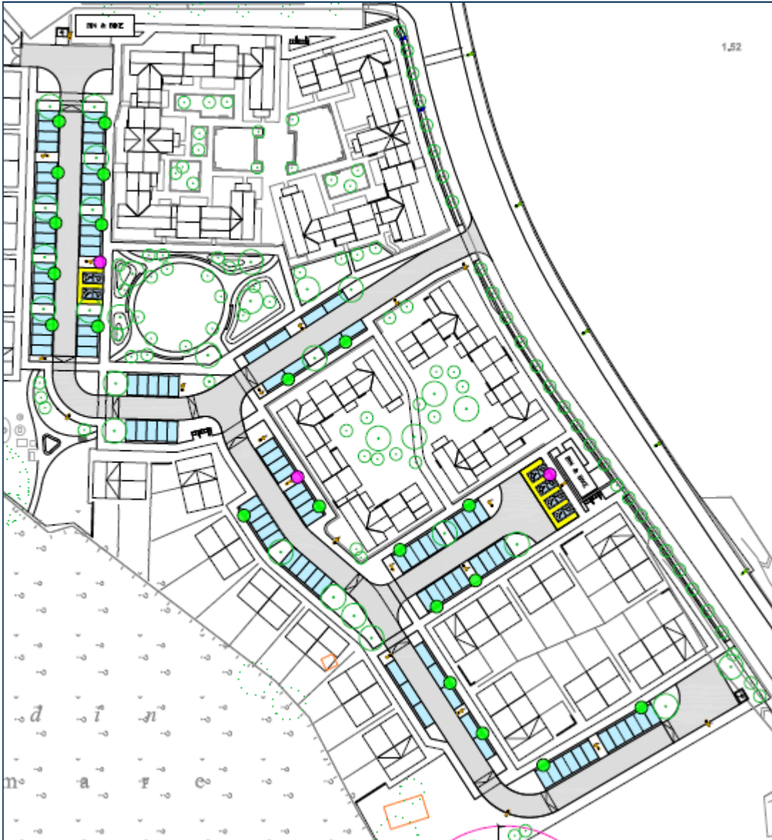
Illustration 5.1: Clip from DKP drawing 80301 with highlighted future ● and operational ● charger point locations.
