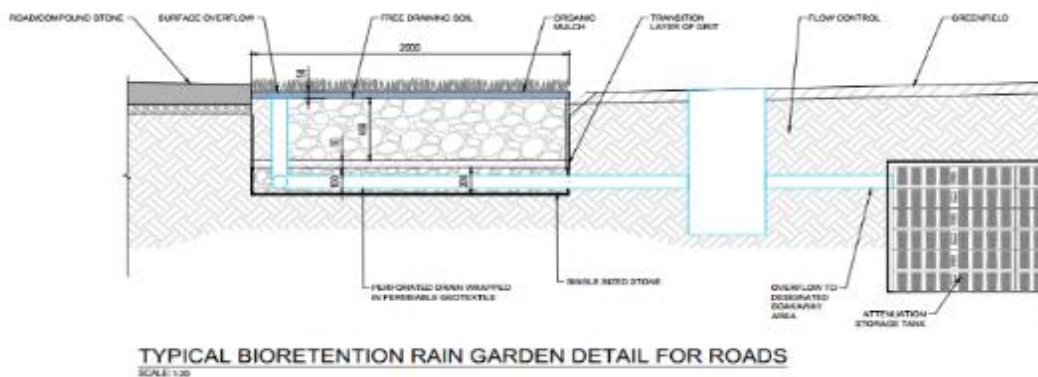
Figure 11: Typical Bioretention Rain Garden Detail (adapted from Drainage Impact Report)
