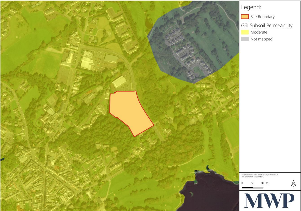
Figure 3-9: GSI Subsoil Permeability
