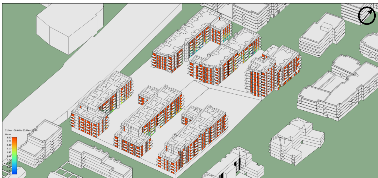
Figure 51: Sunlight Exposure March 21 st (2022 Methodology Medium Level) – SE Elevation
