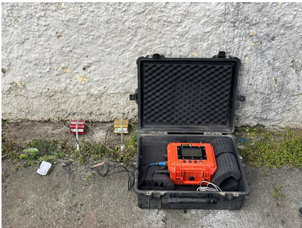
Figure 7: Vibration monitor setup.
