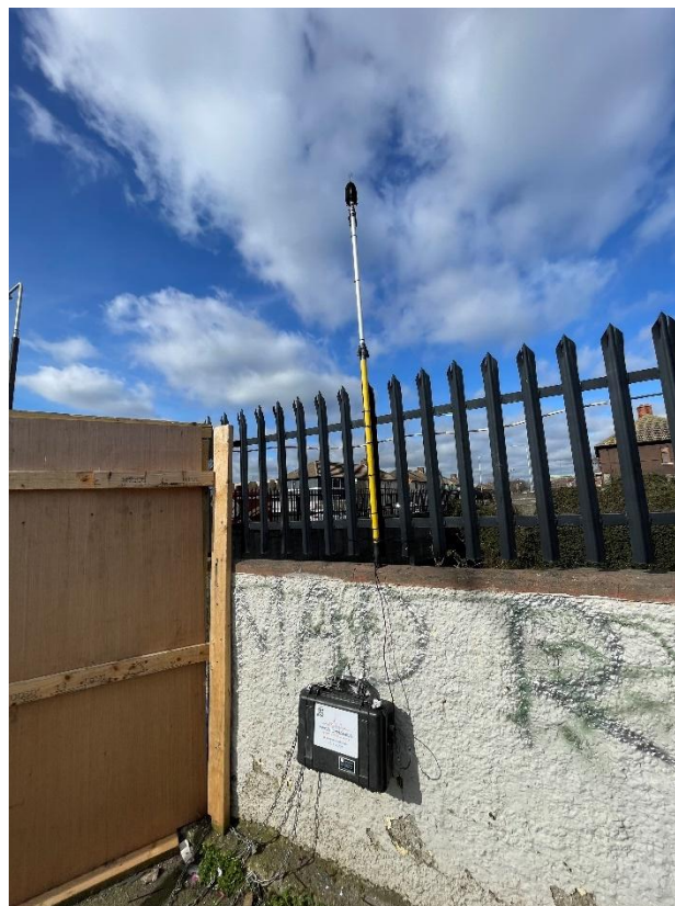
Figure 5: Noise Logger Setup
