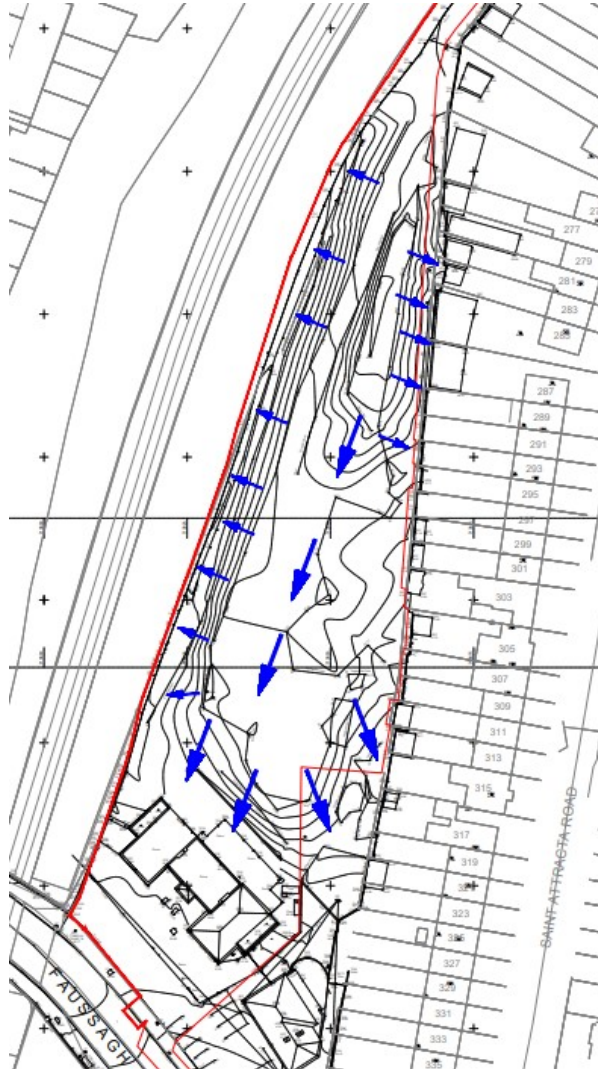
Figure 5.2.3: Existing Flow Routes
