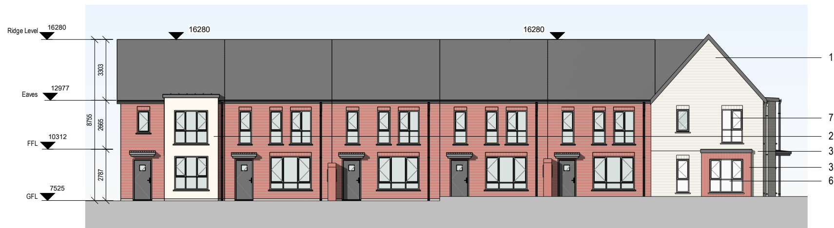
6 Terrace BT72 - Front Elevation Scale: 1 : 200
