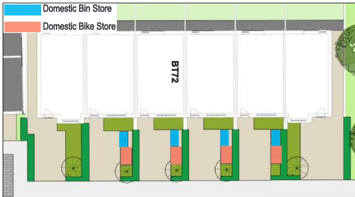
Figure 4-6: In-curtilage Bin / Bike Stores for Mid-Terrace Units
