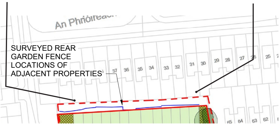
06 Neighbouring Boundary Encroachment
