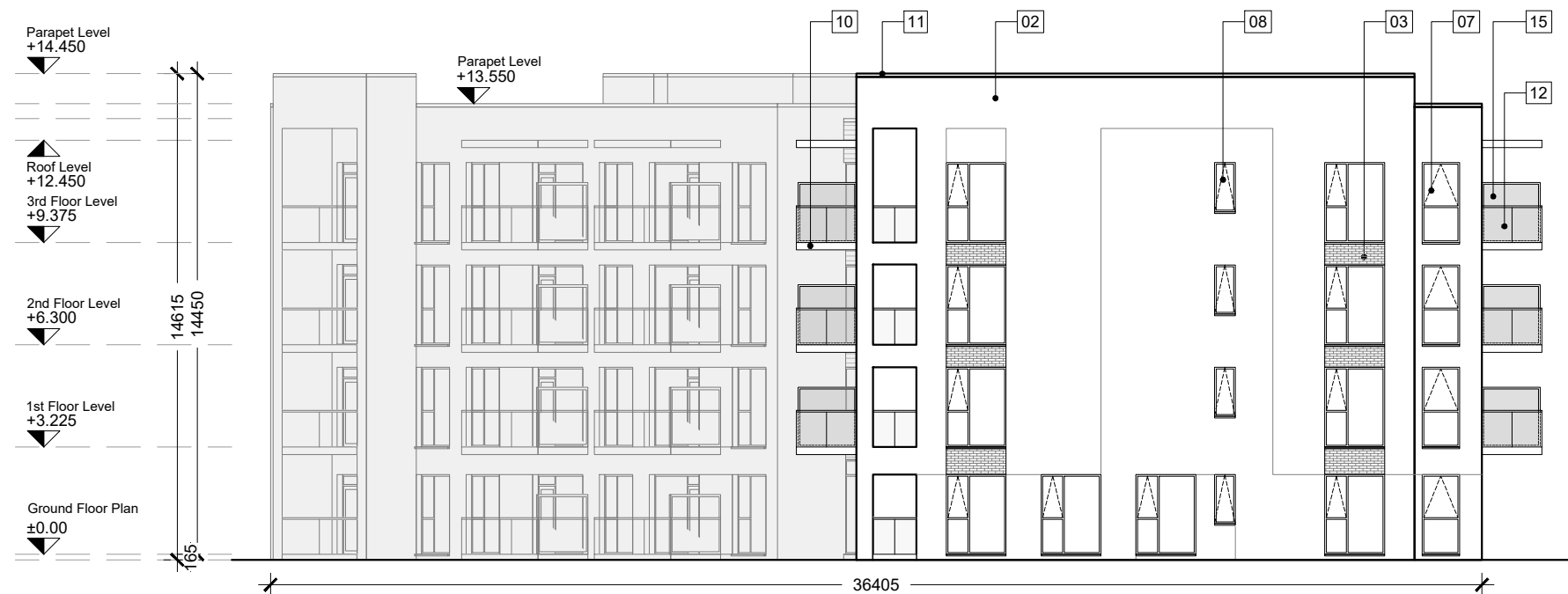
02 Apartment Block A - South-East Elevation (Side) 1:200 @ A1
