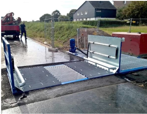
Figure 6.4: Example static wheel wash systems
