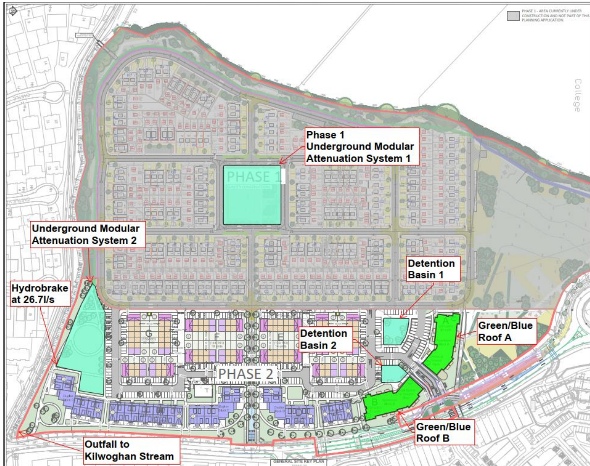
Fig 3.3: Proposed stormwater drainage scheme
