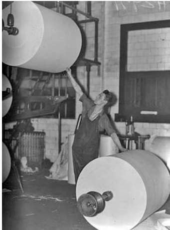
Above left: Webs ready to be loaded into the presses (IND H 2971). Right: The delivery end one of the presses (IND H 2969). Middle:
