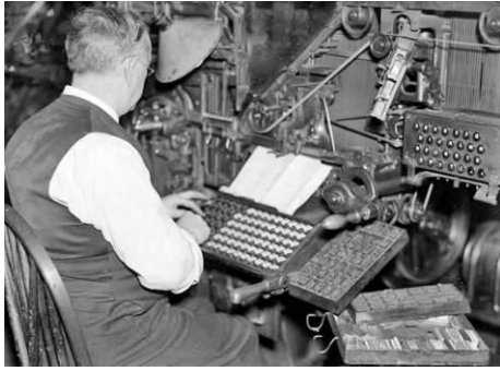
Left: Composing the typeface on a linotype machine (IND H 2967). Middle: Laying out the pages (IND H 2955). Right: A stereotype for loading on to a printing cylinder (IND H 2962).
