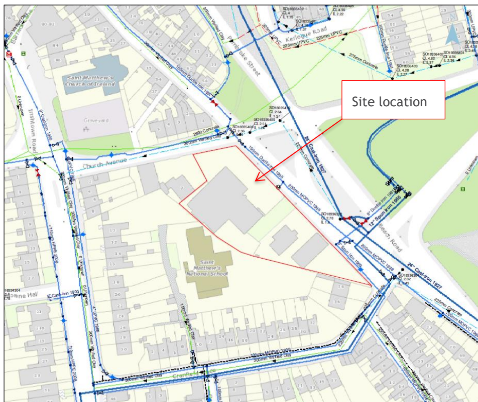
Figure 1: Existing Drainage & Water Mains Surrounding the Site
