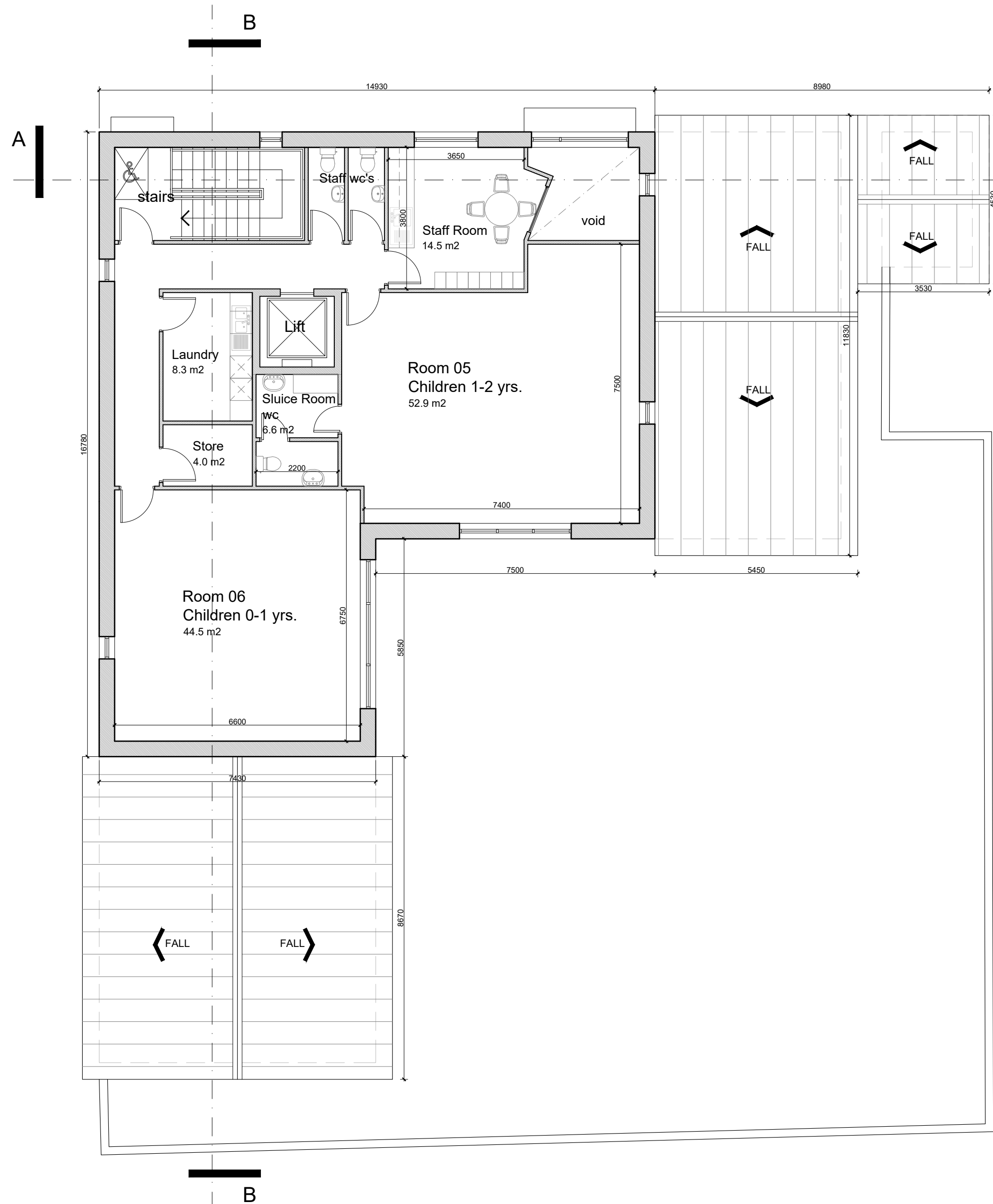
02 FIRST FLOOR PLAN SCALE: 1:100
